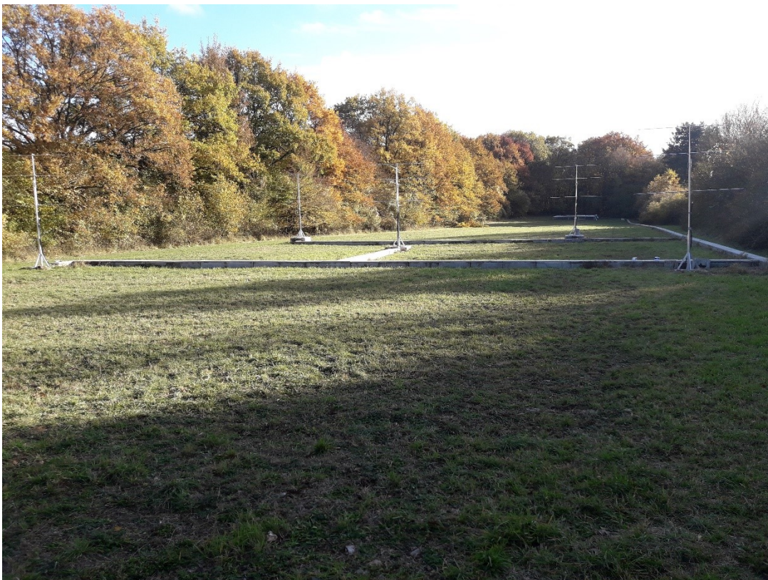
Figure 8: the receiving part of the future meteor radar in Dourbes is an interferometer similar to the one installed in Humain. The transmitter will be an antenna and a grid similar to the BRAMS transmitter and is located in the background at around 200 meters from the interferometer.
